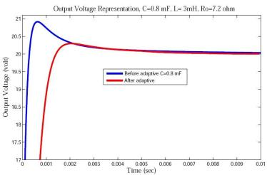
Fig. 11. Voltage responsebefore and after adaptive control of the system after changing capacitance parameter
