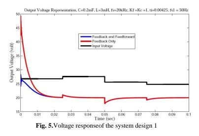
Based on Figure 5, the feedforward design 1 can solve the problem for the first jump in reference voltage, butfor other input jumps this design failed to cancel the effect of the input disturbance.
