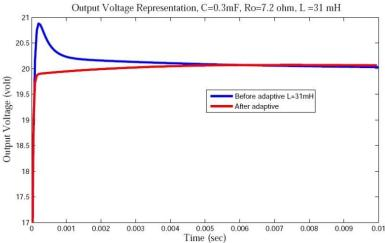
Fig. 10. Voltage responsebefore and after adaptive control of the system after changing inductance parameter
