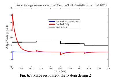
Figure 6 shows that the output voltage of the boostchopper converter is improved in tracking and disturbance
