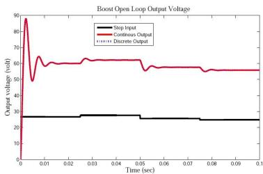
Fig. 4. Continuous-time and discrete-time open loop response of the boost chopper converter
