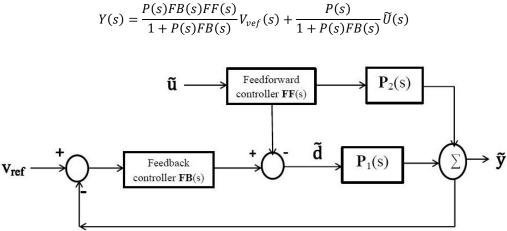
Fig. 3. Boost Chopper System with Both Feedback and Feedforward Controllers design 2
