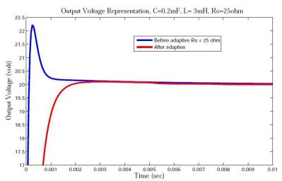
Fig. 12. Voltage response before and after adaptive control of the system after changing resistance parameter
