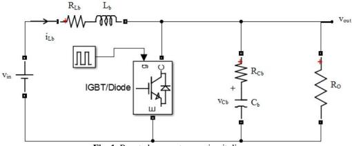
Fig. 1. Boost chopper step up circuit diagram
